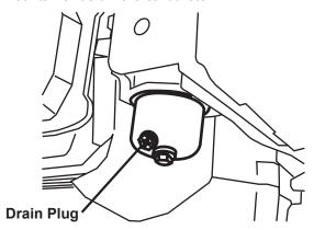
b. Remove the drain bolt from the bottom of the carburetor bowl and allow the fuel to drain.
